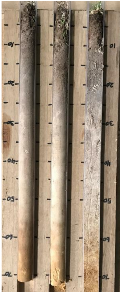
Profile of deep soil cores taken in 2017 showing the organic matter band at 10cm
