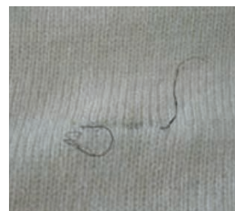
Image: Black polypropylene (Baling Twine) fibre in a fabric. Source: "The Four Pillars of Wool Handling", AWI & Woolmark.
